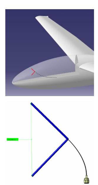
• Alternatively, the following installation with horizontal and vertical antenna legs is also possible.
