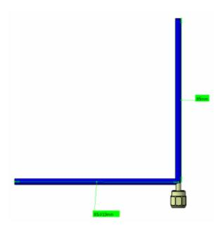
• The following applies to the *FAnt* or *RAnt* : The two legs of the antenna should lie along a line and be vertical.
